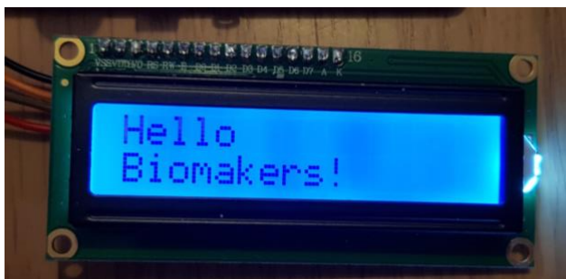
I2C 1602 LCD Display Module Programmed to Show Text
