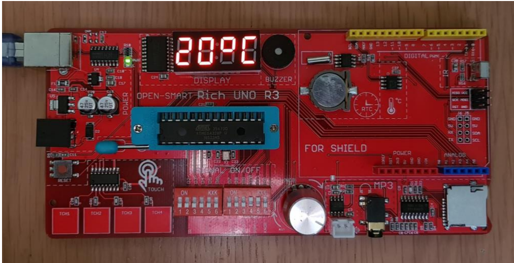
Arduino Rich Uno R3 Board Displaying the Temperature in °C
