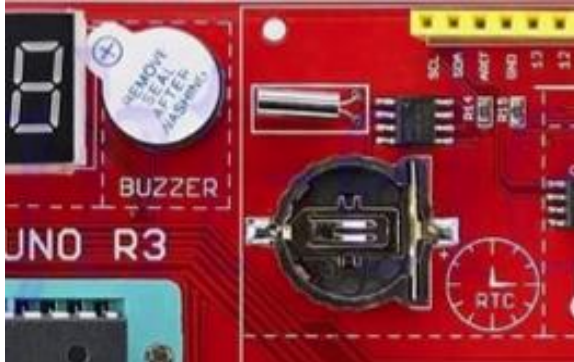
Real Time Clock (RTC) Module on the Arduino Rich UNO R3 Board
