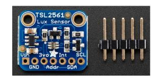
Connect using expansion shield or Grove-to-female wires (make sure pin labels match up)
